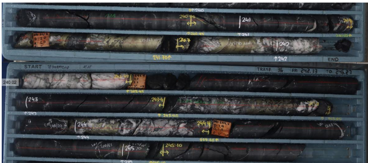
Figure 3: DD24KP1208 intersected 3.08m @ 3.1g/t Au, 4.1% Cu, 30.3g/t Ag from 241.31m. Mineralisation is hosted within a quartz vein with prominent sulphides including 2-20% chalcopyrite, and 1-5% pyrite.
