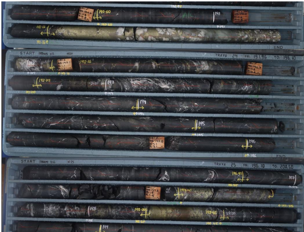
Figure 4: DD24KP1212 intersected two mineralised structures within a 7.29m zone of anomalism from 191.16m, reporting 2.6g/t Au, 3.1% Cu, 16.4g/t Ag – inclusive of internal dilution > 1m. The significant intersections reported within this interval are 1.59m @ 8.5g/t Au, 8.2% Cu, 24.8g/t Ag from 191.16m and 1.04m @ 4.5g/t Au, 8.8% Cu, 73.9g/t Ag from 197.41m. Mineralisation is hosted within a quartz vein with prominent sulphides including 5-20% chalcopyrite, and 2-5% pyrite.
