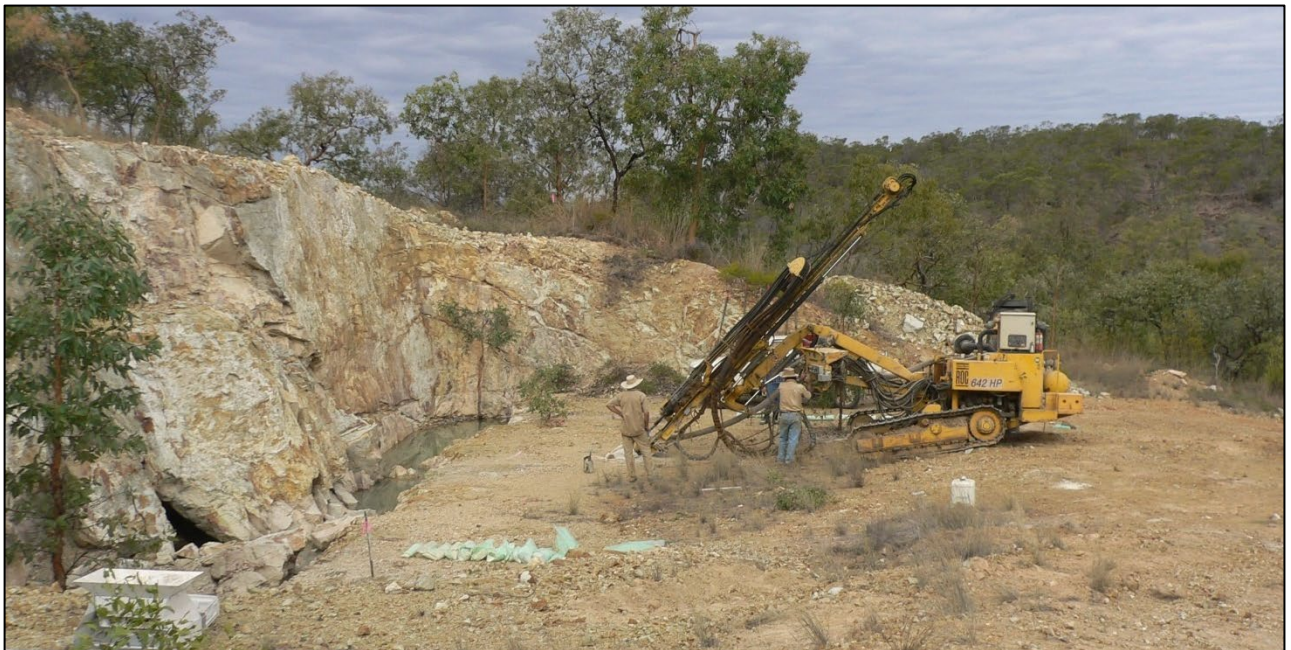
Figure 3: Shallow airtrack drilling beneath the 1991 trial pit at Francis Creek (from CR40465, 2005).
