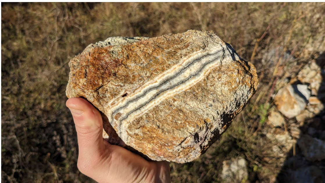
Figure 5: 2cm wide colloform-crustiform banded vein from Francis Creek comprising of quartz, adularia and marcassite (approx. 10%).
