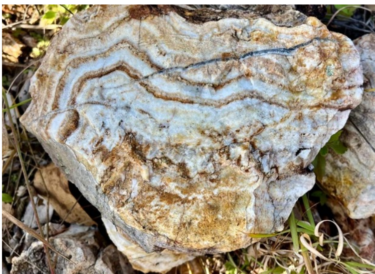
Figure 1: An example of colloform banded veining from Francis Creek with later 5mm adularia-marcasite (est. 20% of vein) veining cross-cutting the banding. Sample was slabbed and sent for assay.
