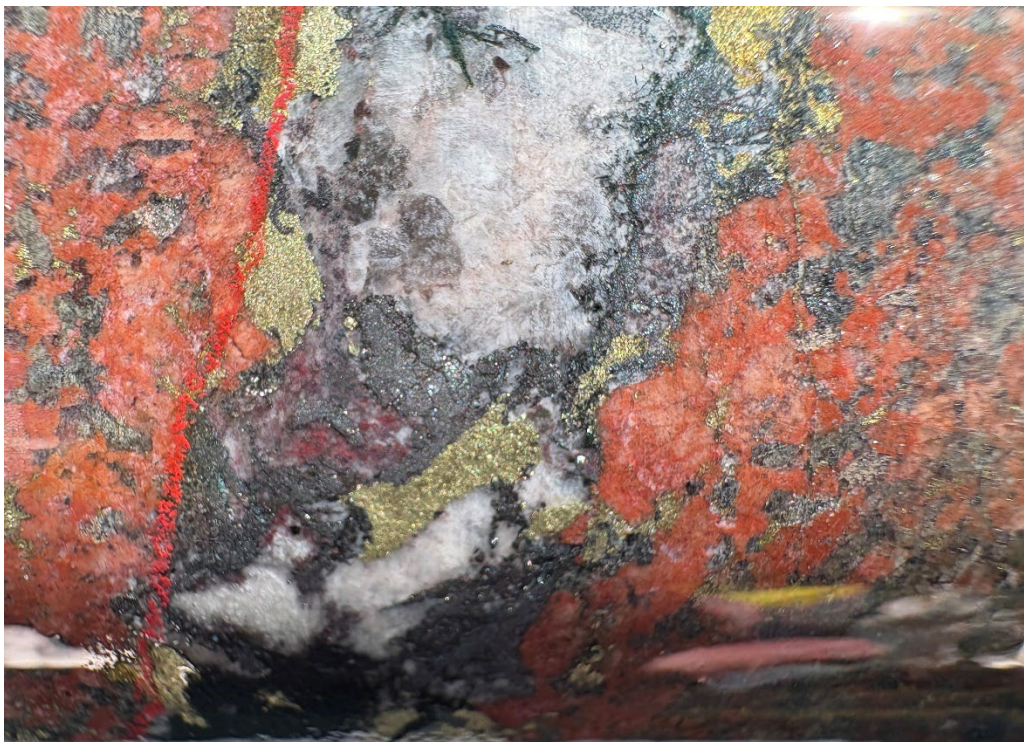
Figure 6. HMBDD003, ~474m. Calcite, magnetite, hematite vein with pyrite and chalcopyrite.
