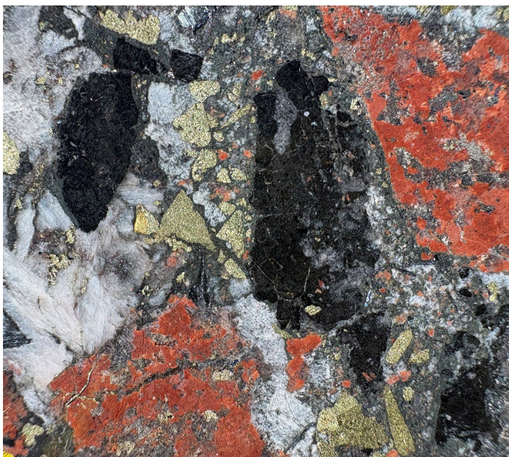
Figure 3. HMBDD003, ~331.4m. Vein breccia. Strong red rock altered protolith with carbonate, specular and earthy hematite, biotite, pyrite and chalcopyrite. Down-hole is to the right.
