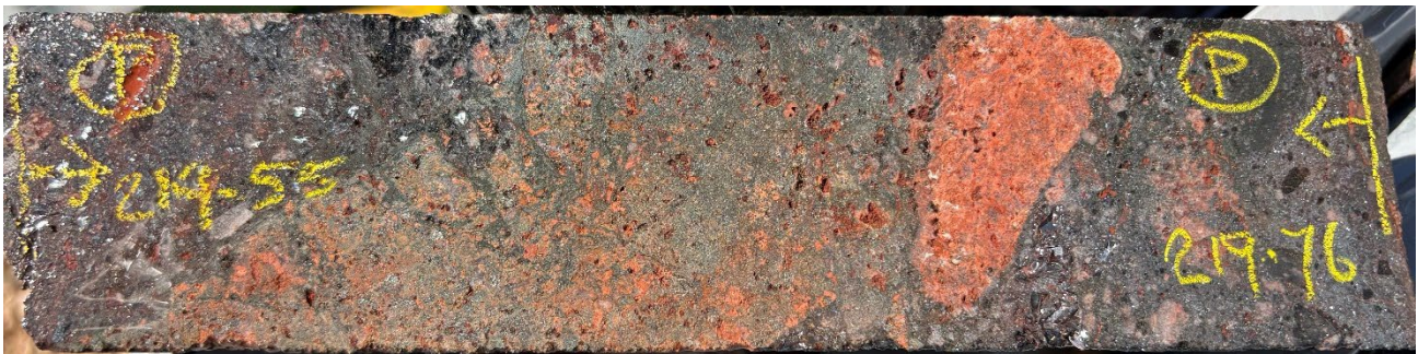
Figure 5. HMBDD003, ~219.6m. Vein breccia in altered granite with earthy hematite after an unknown mineral in clasts. Down-hole is to the right.
