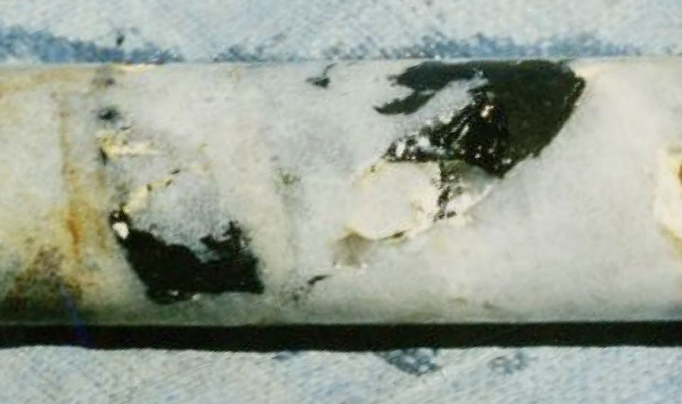
Coarse Wolframite (left) and Molybdenite (right) in NQ Diameter (47.6mm) Drill Core from Glen Eden diamond drill hole GENS81-5 (Source - ASX release 2 July - Amoco 1981, depth not recorded. ).
