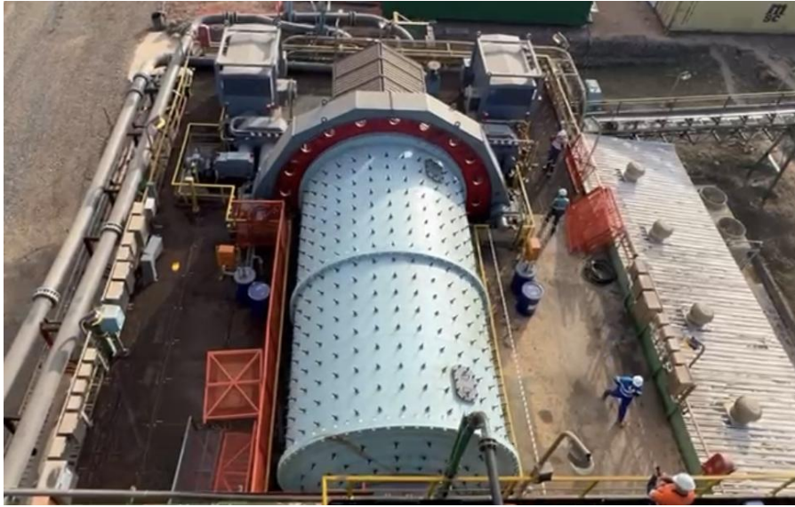
Figure 1: SAG mill refurbishment completed
