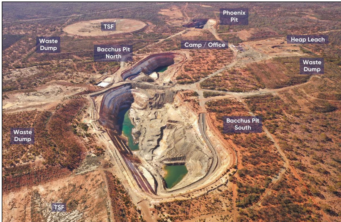
Figure 2: Historical pits, rehabilitated leach pads and waste dumps, tailings storage facility and camp
