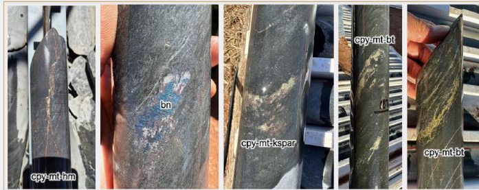
Observations from hole 24WADD002 drill core showing IOCG-style mineralisation including magnetite +/- hematite (mt, hm), boronite (bn), chalcopyrite (cpy), potassic feldspar (ksp) and biotite (bt). Visible gold was also observed. 4
