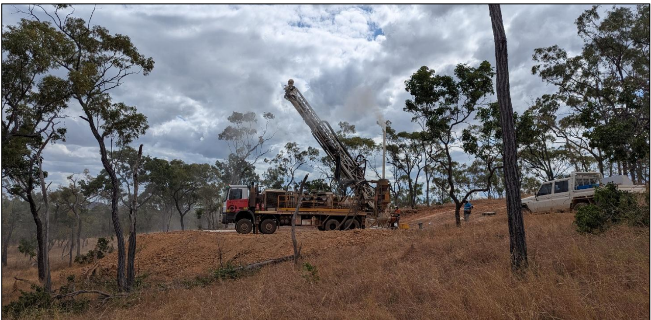
Figure 1. Reverse circulation drilling underway at the Bouncer Prospect.
