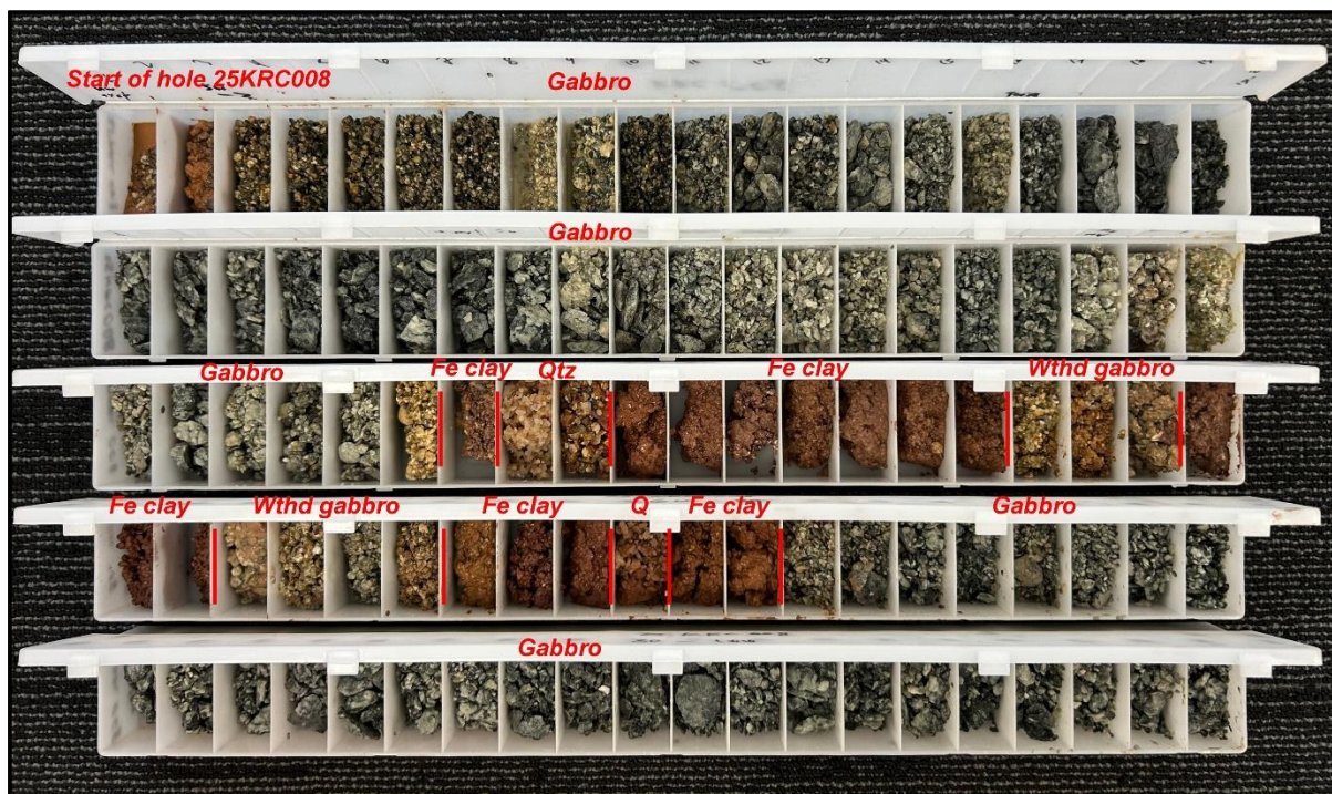
Figure 5: Drillhole 25KRC008 chip trays showing heavily weathered ferruginous material and quartz downhole
