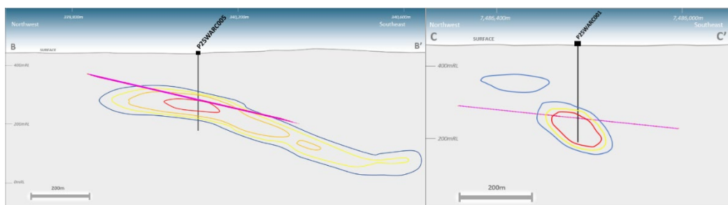
Figure 7. Maton B (B-B' left) and Maton C (C-C' right) cross-sections with planned drillholes Modelled AEM conductor source body plates and conductivity inversion model iso-surface shells
