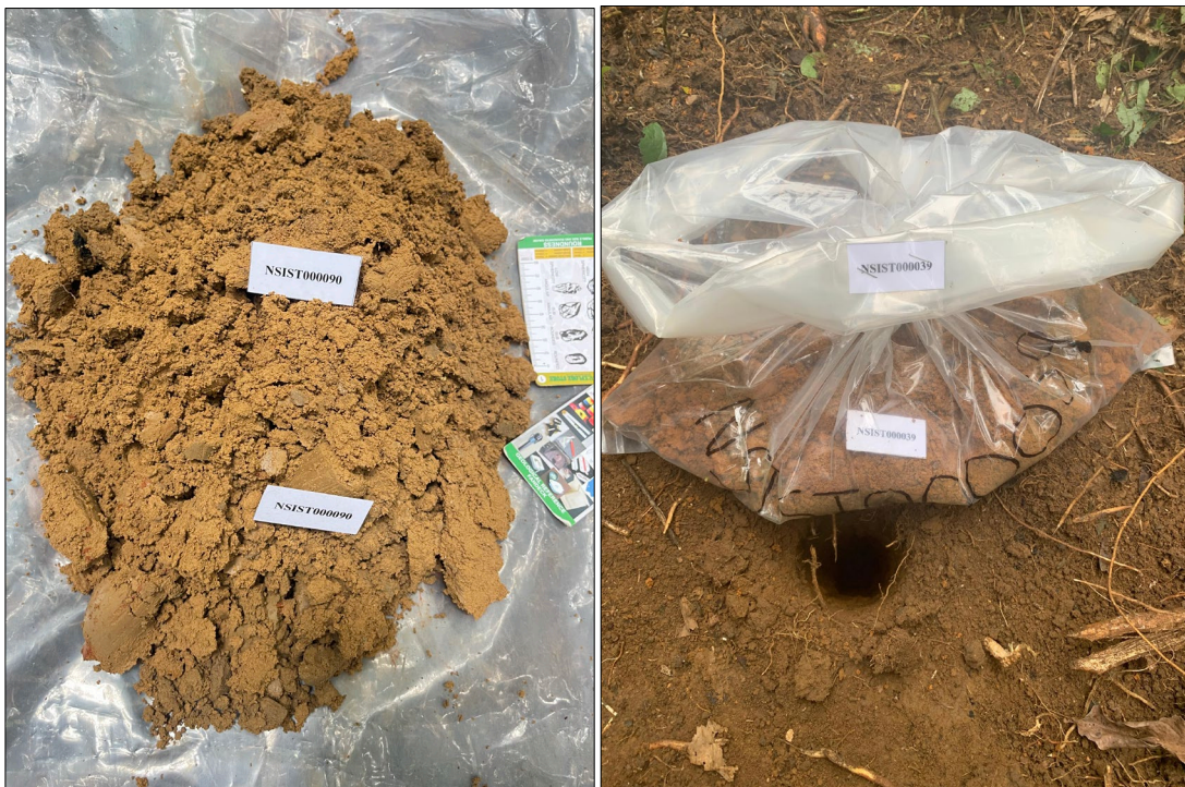
Figure 4: A freshly collected soil sample being logged along with a bagged and tagged sample next to the sampling point.
