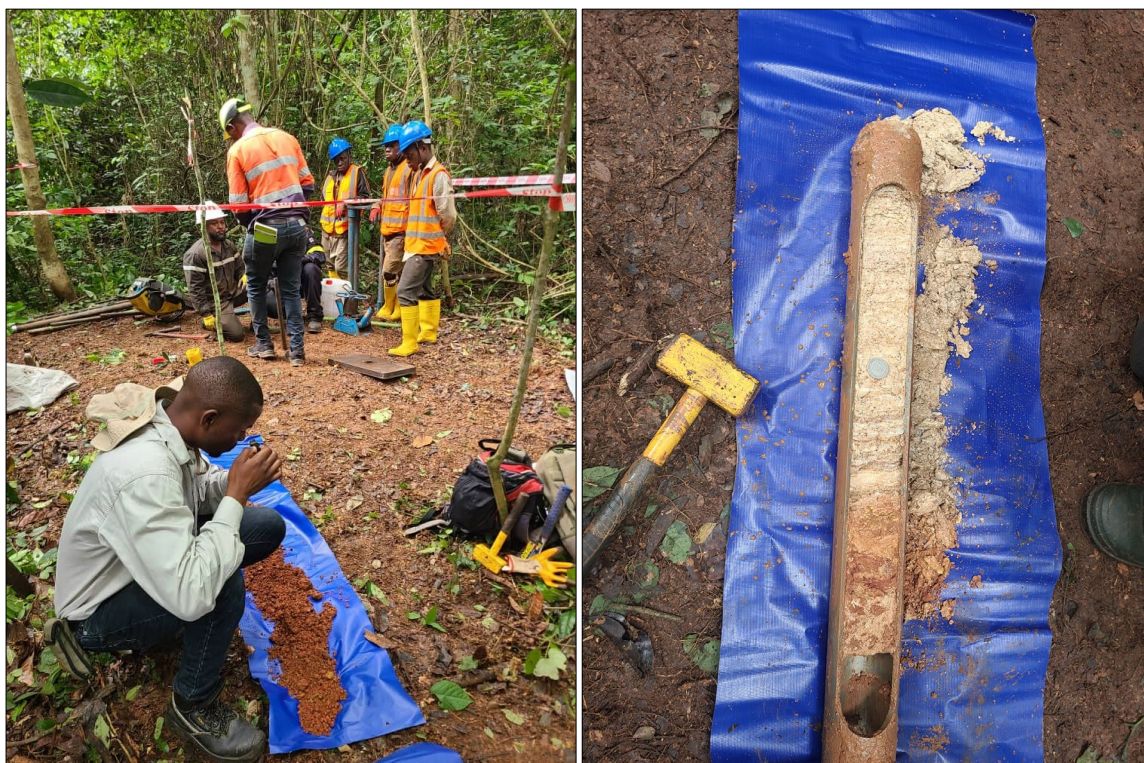
Figure 2: DY6 Project Geologist Geoffrey Banda logging drilling samples, along with a freshly drilled saprolite intercept from 8 to 9m.
