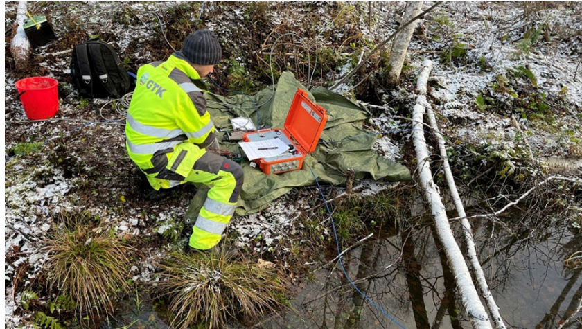
Figure 10: Installation of magnetotelluric measuring equipment
