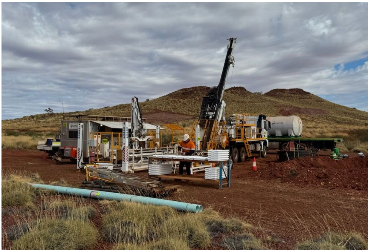
Figure 10: Diamond drill rig on pad 25BKDD001 at the Barkley gold target
