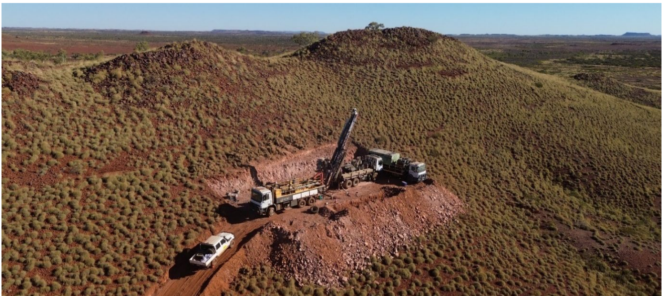
Figure 1: RC drill rig on pad at 25BKRC009 at the Barkley Gold target
