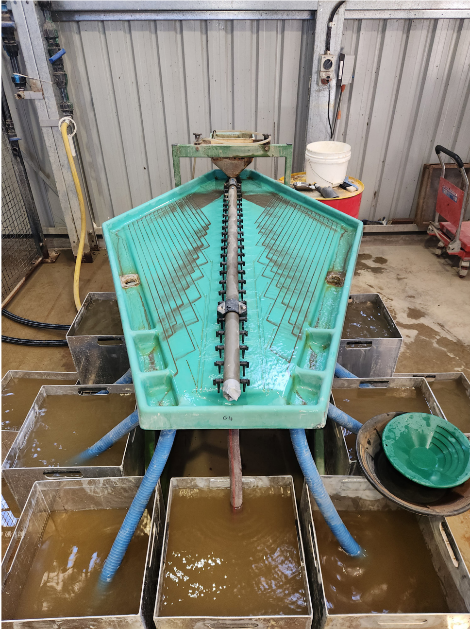
Figure 2: Gemini table refining gold in sulphides concentrates.
