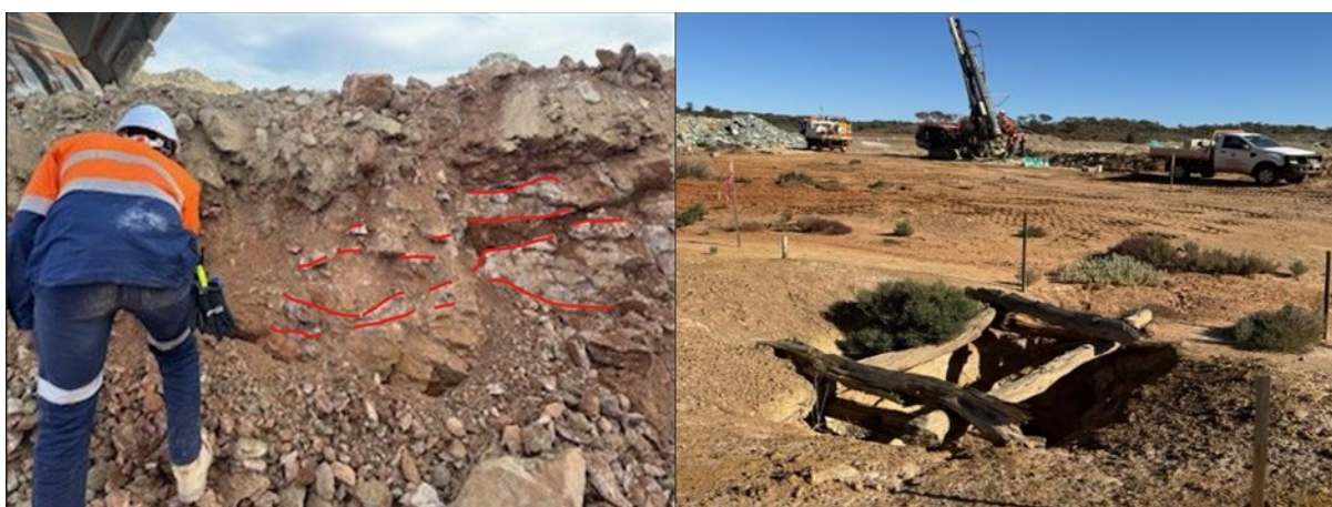
Plate 7 Mapping the ore structure (left) and (right) drilling along strike of 1920s mining shafts
