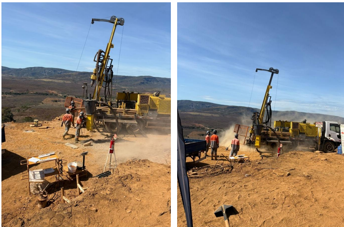
Figure 2: Image showing Reverse Circulation (RC) drilling underway at “Target 1” at the Igrejinha Lithium Project.
