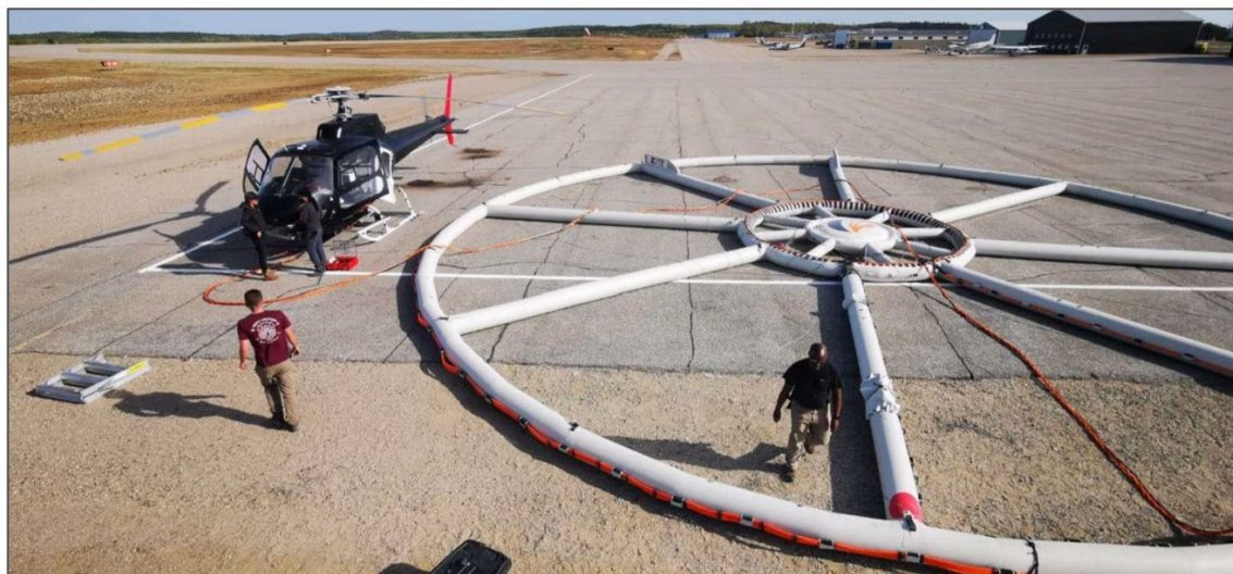
Figure 6: Configuration of Xcite™ TDEM survey system.
