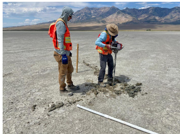
Figure 10: Auger Sampling at White Plains Lithium Brine Project, Utah, USA
