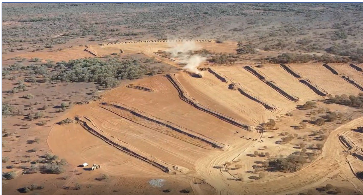
Figure 2: Initial open pit works commencing at Trident; the open pit is intended to take 12 months before commencement of the underground mine
