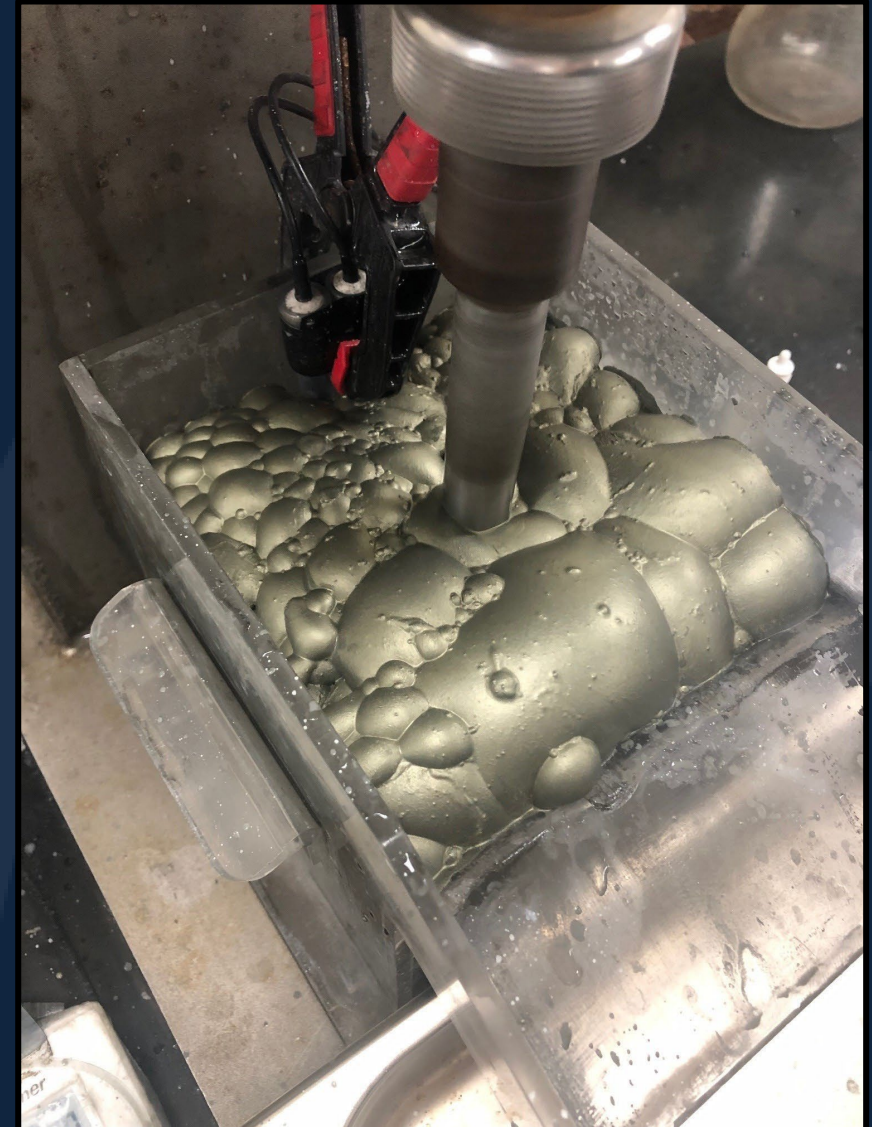
Sulphide flotation of Callisto sample from NRCD337
