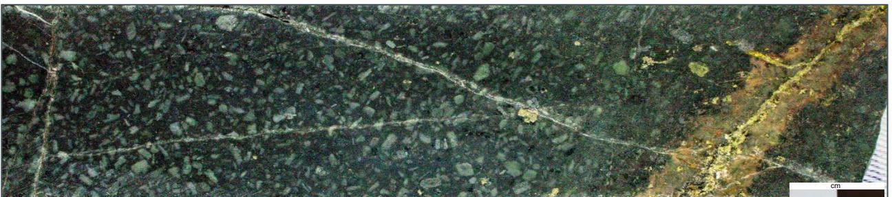
SPRCD062 - 669.7m – Veinlet chalcopyrite + quartz ± pyrite with strong k-feldspar vein halo, 43.3g/t Au
