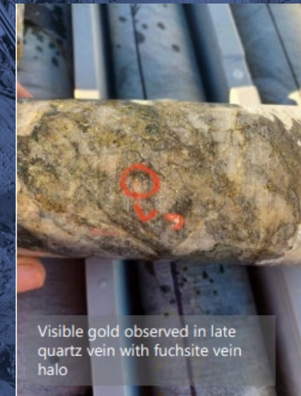
Visible gold observed in late moderately south dipping quartz vein with fuchsite vein halo
