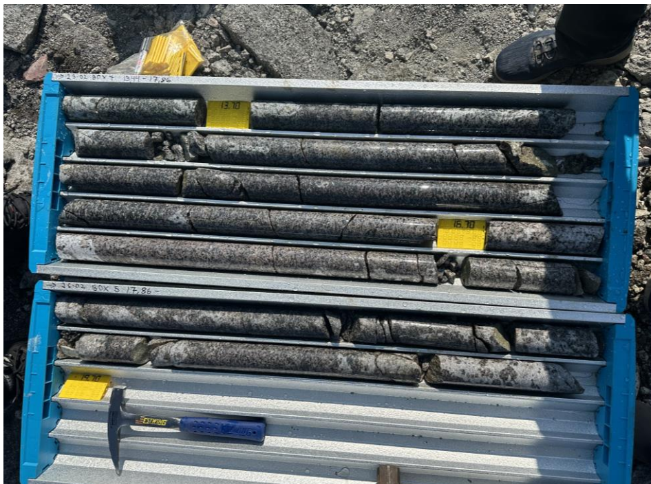
Figure 7 - 2025 diamond drill hole drill core DDH25-02, close up showing mauve eudialyte
