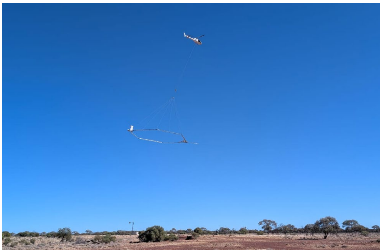
Figure 1 – Helicopter with SkyTEM system flying grid pattern over Marymia East tenements
