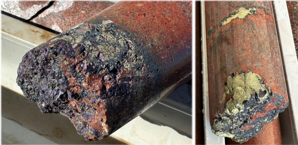
Left: 424.05 – 425.10m (bornite &+chalcopyrite). Right: 567.35 – 567.45 (massive chalcopyrite)
