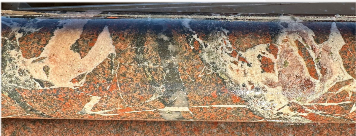
530.5 – 530.6m Breccia with k feldspar and hematite alteration.
