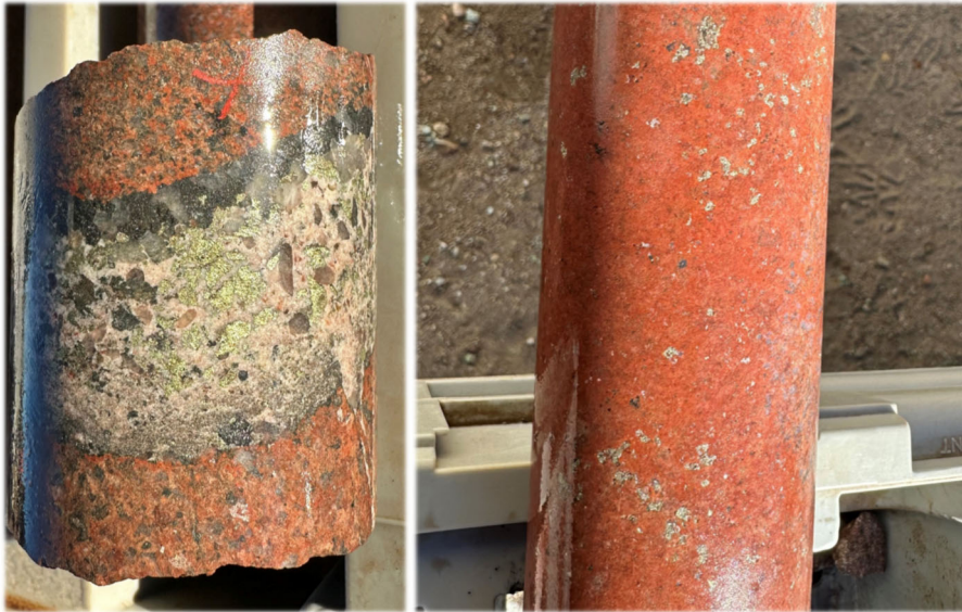
Left: 564.3-564.4 Vein hosted chalcopyrite. Right: 607.5-607.6m disseminated chalcopyrite.
