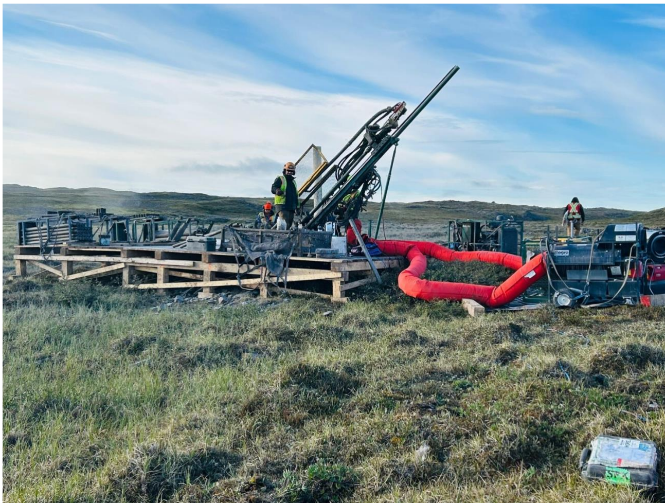
Figure 2 - Reverse circulation drilling underway at DAN25019.
