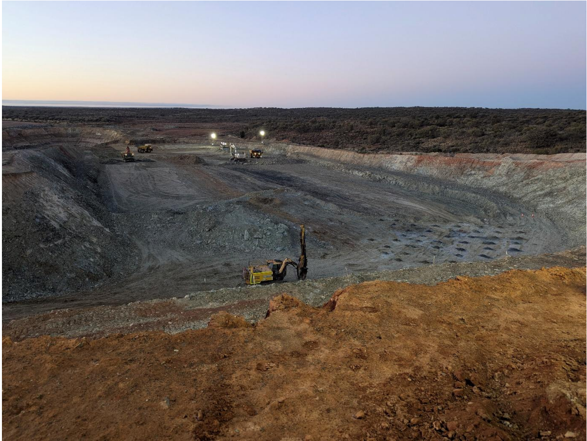
Visual ore (brown streak) marked out in the Devon Pit floor between grey waste rock (7 August 2025)
