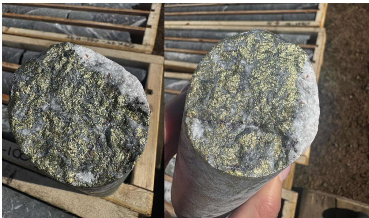
Figure 4 - Example of chalcopyrite-bornite-quartz-carbonate veining within the Husky Creek Formation of STK25001 at 291.4m. Core diameter is NQ2. Cautionary Statement: The Company cautions that, with respect to any visual mineralisation indicators, visual observations and estimates of mineral abundance and uncertain in nature and should not be taken as a substitute or proxy for appropriate laboratory analysis. Visual estimates also potentially provide no information regarding impurities or deleterious physical properties relevant to valuations. Assay results from the drilling and sampling programmes will be required to understand the grade and extent of mineralisation. Initial assay results are expected in the September quarter.
