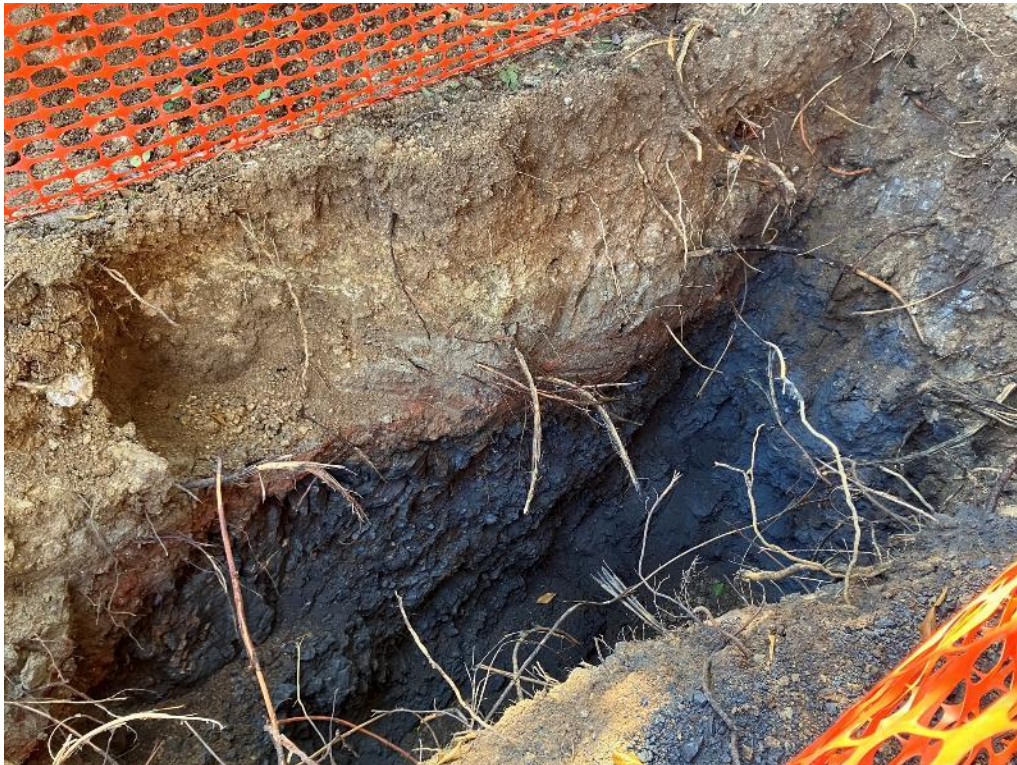
Trenching at Ira Miri showing 95% Manganese Oxides - See ASX Announcement dated 3 June 2025 and Visual Estimates Cautionary Statement in the disclaimer
