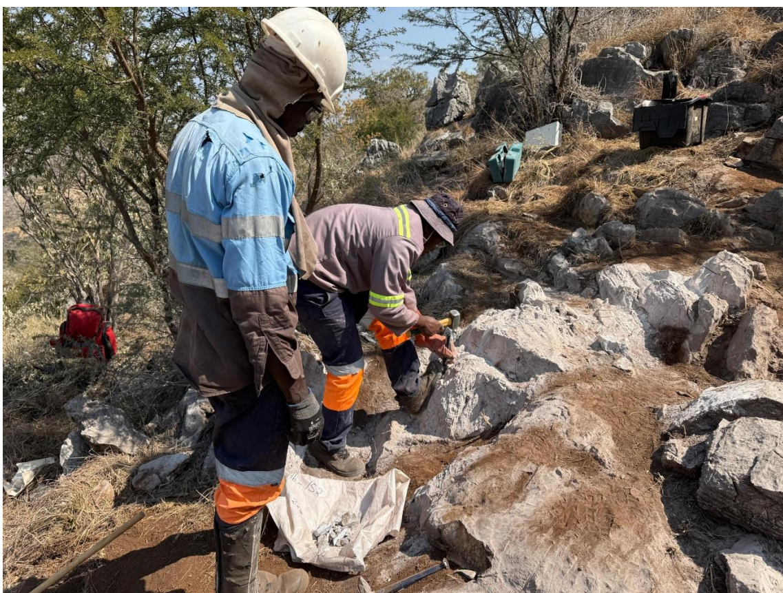
Image 3: Graceland Prospect, Golden Deeps field personnel, channel sampling across the Gossan/Sulphide 2 outcrop
