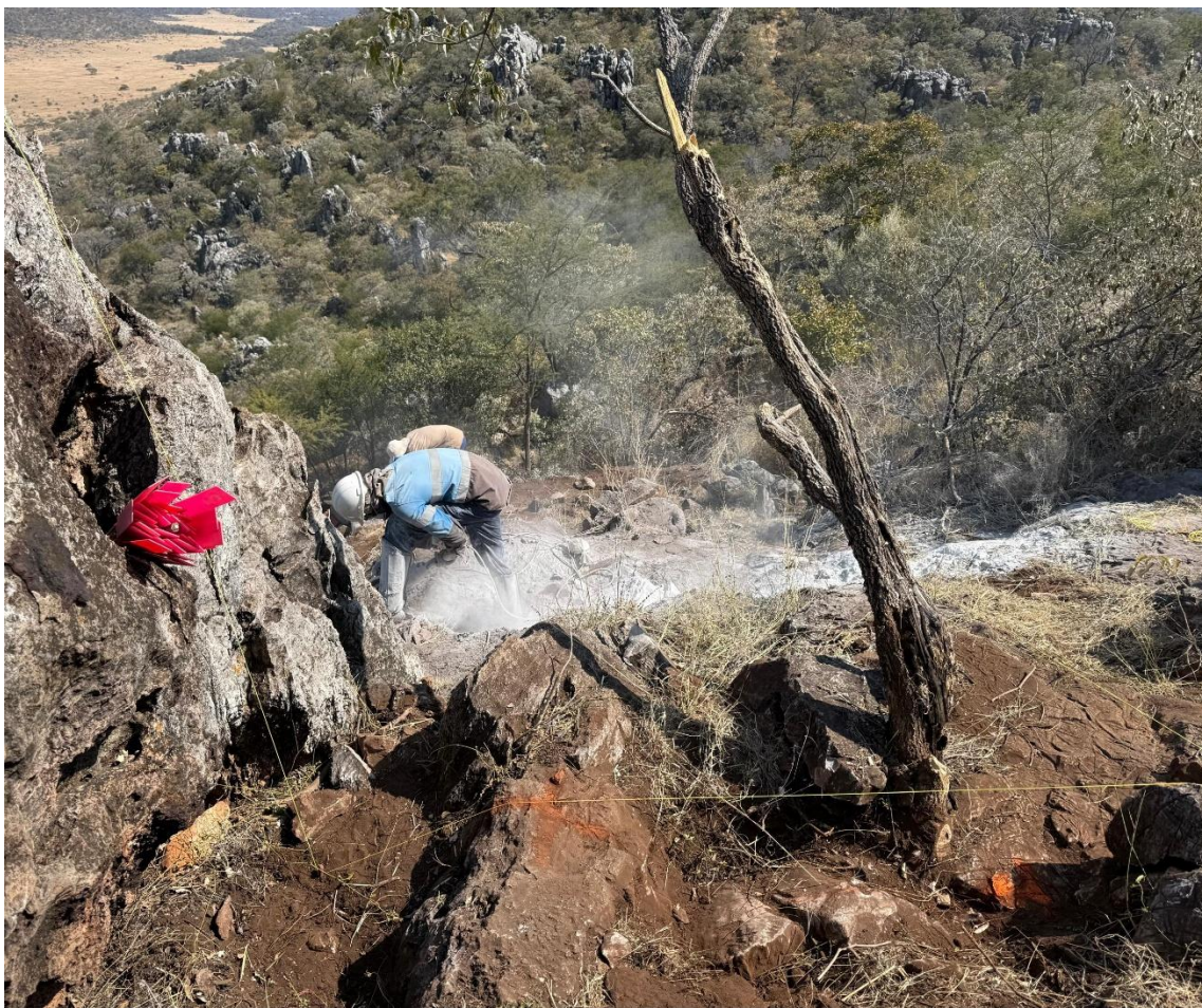
Image 2: Graceland Prospect, Golden Deeps field personnel, diamond-saw channel cutting across the Gossan 1 outcrop
