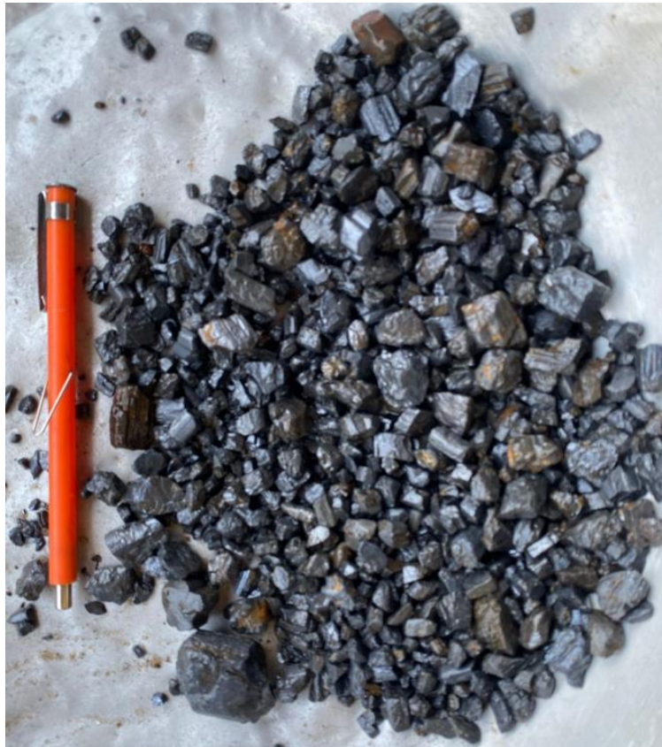
Figure 1: Image of nuggets from sample MRGR0023 with rutile grading 98.6% TiO 2 .
