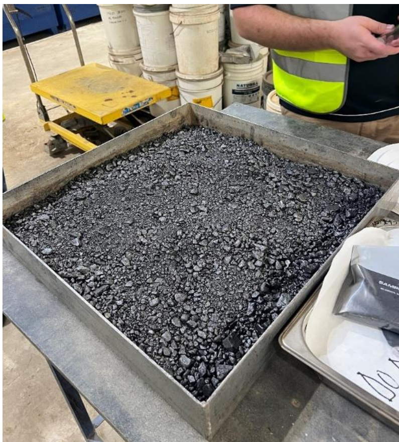
Figure 1: Graphite concentrate (93.4% graphite) sample used in purification tests
