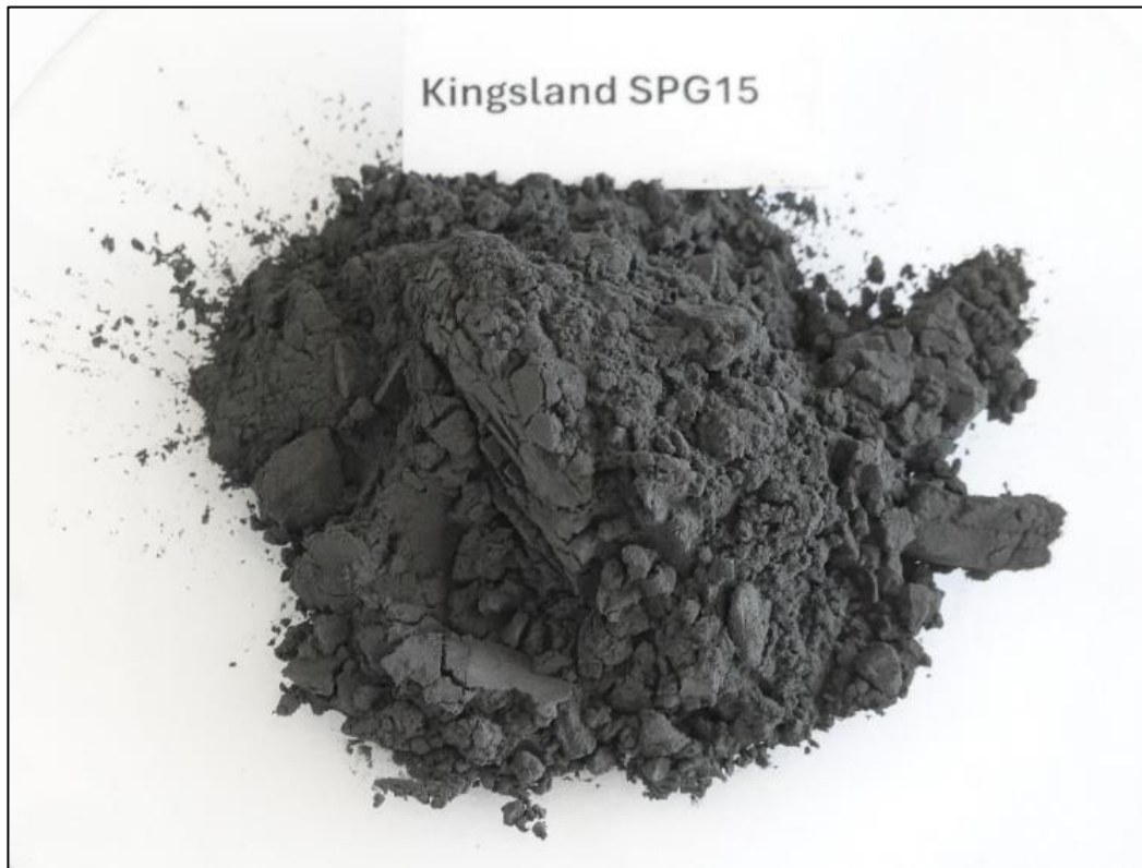
Figure 2: Sample of Spherical, Purified Graphite (PSG) >99.95% graphite, generated from Leliyn concentrate
