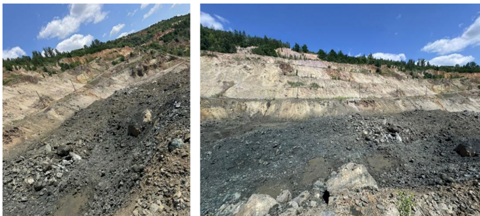
Image 2 and 3: Blasted Graphite Ore ready for Loading and Hauling to the ZG ROM Stockpile
