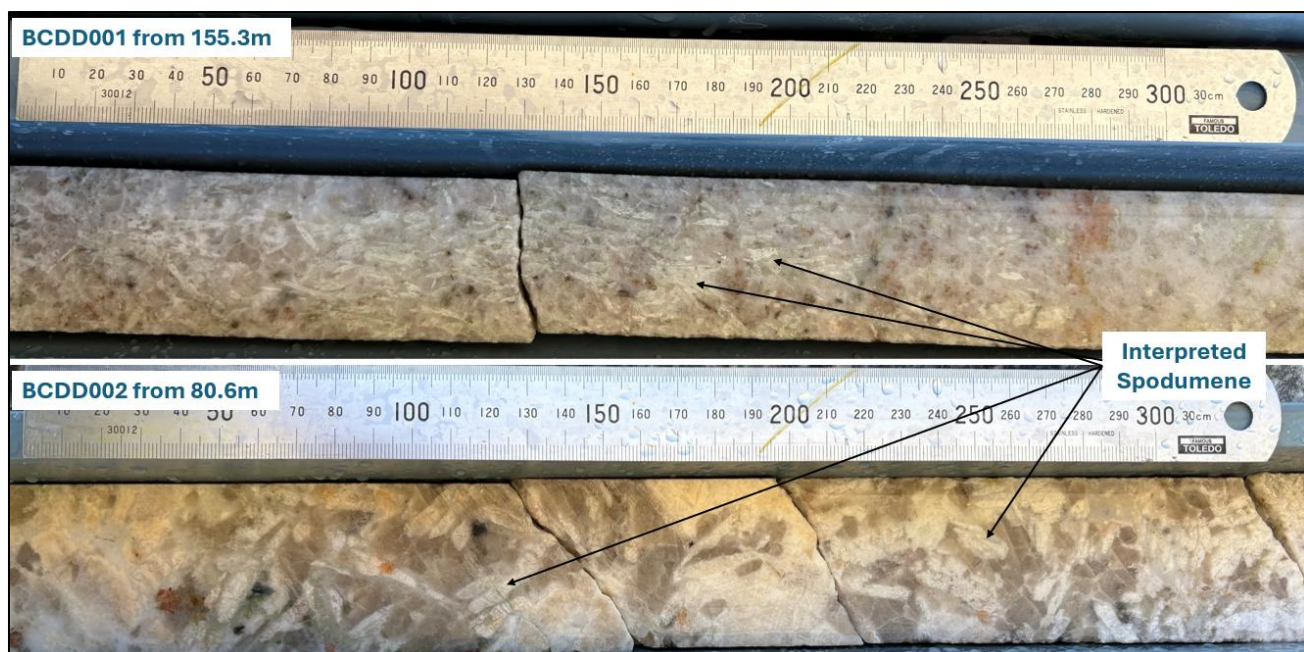
Figure 3: Top : Cut diamond core sample from BCDD001 starting at 155.3m. Abundant slender white elongate crystals are likely spodumene. Bottom : Cut diamond core sample from BCDD002. Large white crystals are likely spodumene. Estimated spodumene abundance is ~40% in both intervals.
