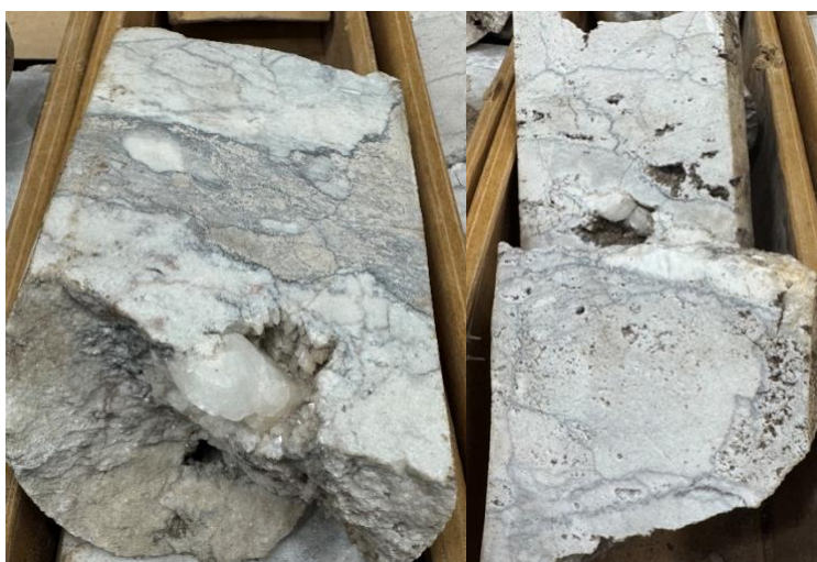
Photo 1: Example of diamond core showing fracturing & vugs in the extraction horizons.
