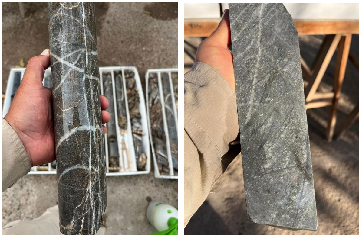
Figure 1 (left image): IE-001-2025 drill core from 177 to 180 metres showing potassic alteration and stockwork. Visually estimated grade 0.1 - 0.4% Cu. Laboratory assay results are due to be received in September 2025.
