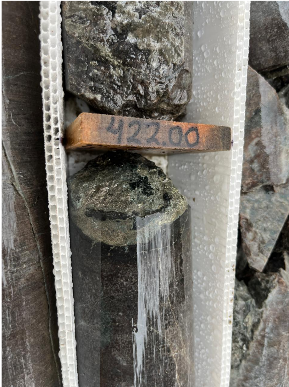
Figure 3: IE-001-2025 drill core at 422 metres displaying sulphides in quartz veining in granular diorite. Visually estimated grade 0.1 - 0.4% Cu in dissemination. Laboratory assay results are due to be received in September 2025.
