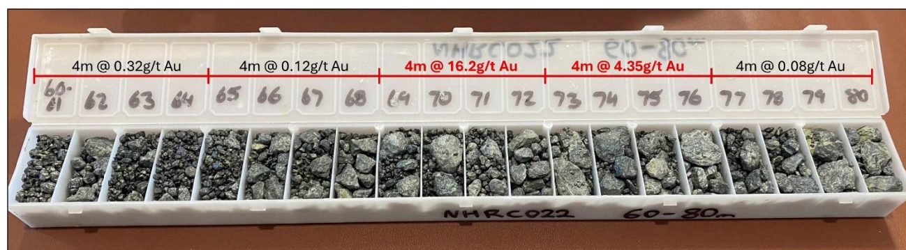
Figure 2: RC drill chips from 60m to 80m down hole depth from NHRC022 with mineralised intervals
