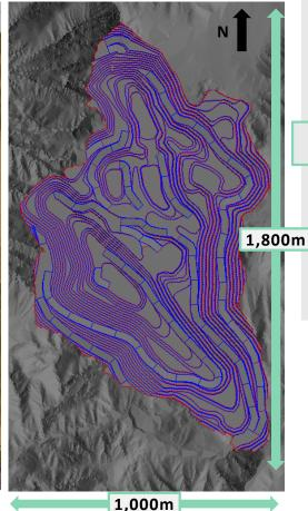
DFS considers 8 phases of pit development to provide consistent ore feed to the heap leach
