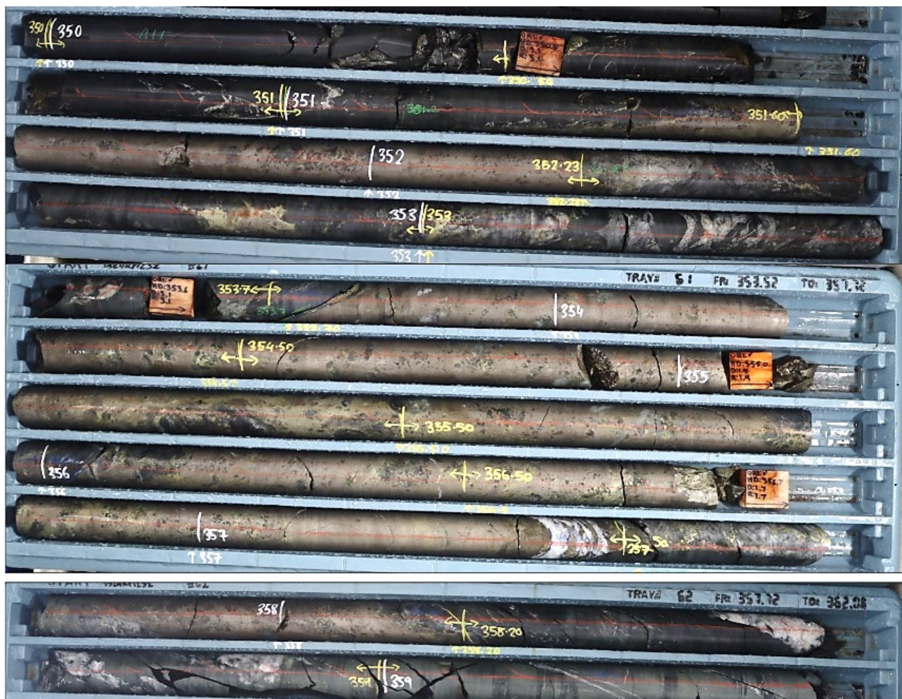
Figure 3: Mineralisation occurs as massive and semi massive sulphides overprinting quartz veining from 351.2m, comprised of pyrrhotite (60%) and semi massive chalcopyrite (15%) and pyrite (5%). True width of the interval is estimated to be approximately 65% of the visually logged intercept length.
