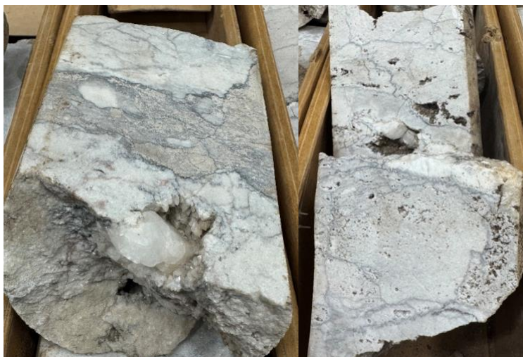
Photo 1: Example of diamond core showing fracturing & vugs in the extraction horizons.
