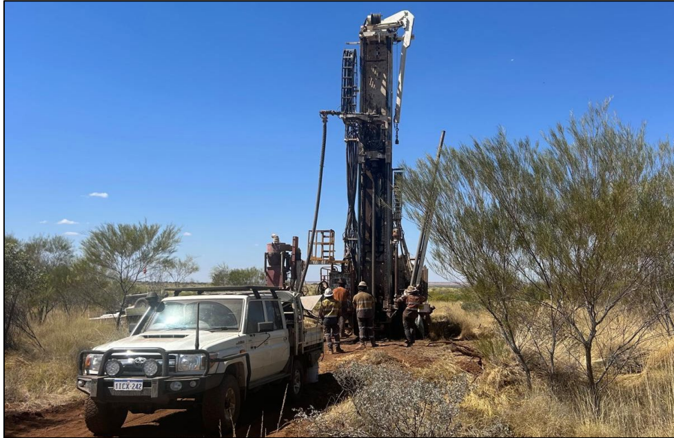
Figure 1: RC drill rig on tenement E46/1407 collaring into the manganese formation looking to the east.
