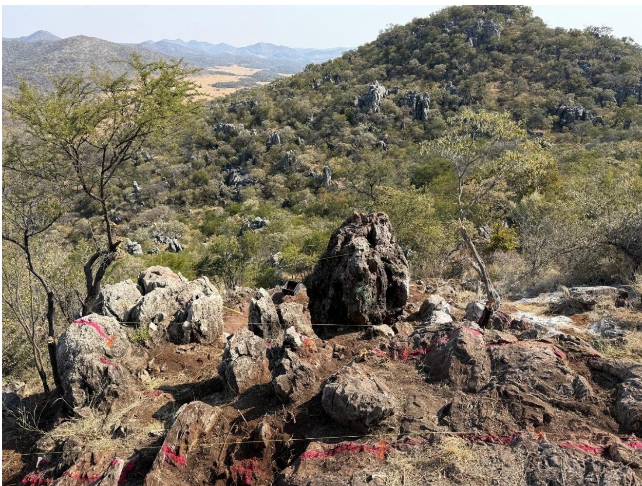
Image 1: Graceland Prospect, Gossan 1 – showing channel sample lines prior to sampling of the mineralised zone
