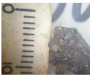
Photo of rock chip from hole TGRC23004, 117-118m sample interval with reported grade of 7.8g/t Au<sup>2</sup>. Scale on left is in millimetres (mm). See ASX Release 19 September 2023 for more details
