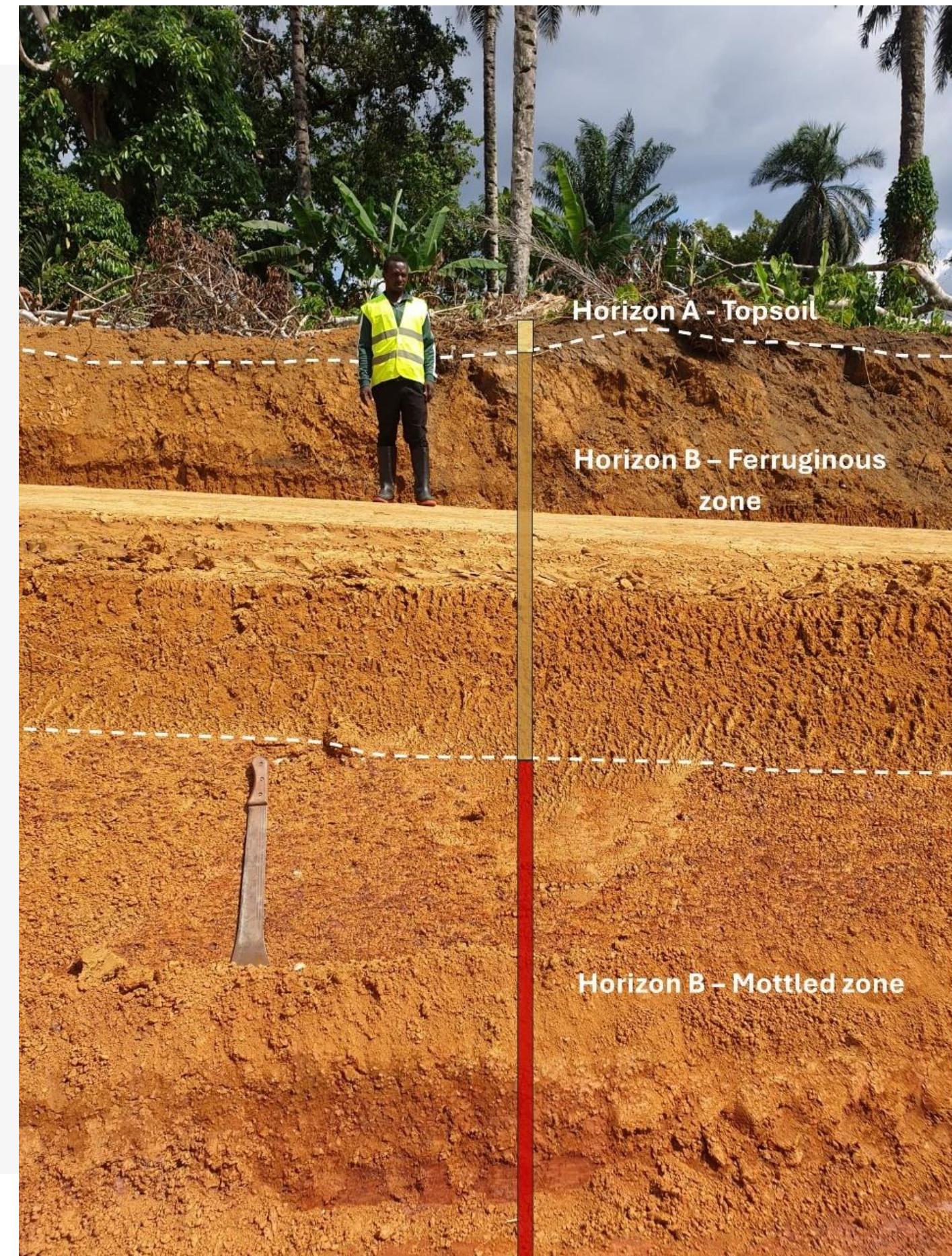
Figure: Weathering profile at the Bounde licence showing a classic residual “Kasiya-type” profile
