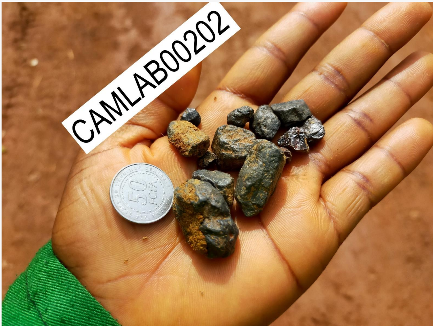
Figure : Rutile nuggets from the Bounde licence grading 96,74% TiO 2 (refer to announcement on 11 August 2025 “XRF analysis confirms high quality of natural rutile”)
