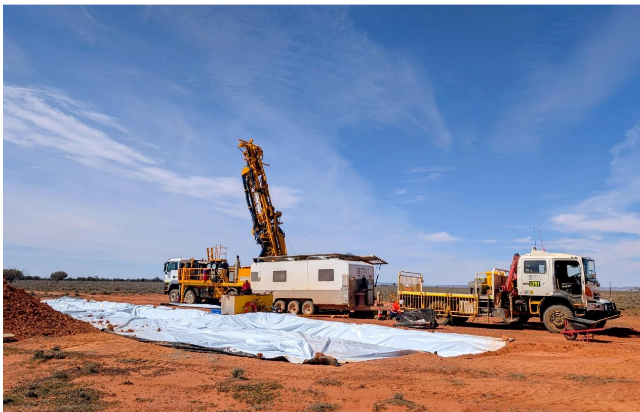
Figure 1: The diamond drill rig setup at the Woolly target on drillhole 25WLDD0001
