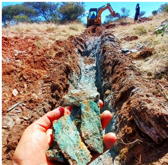
Photo 1 (left): Copper oxide mineralisation in schist at the South Otavi Project – DET003 2-5m Photo 2 (right): Copper oxides within ferruginous-calcite at the South Otavi Project – DET003 61-62m
