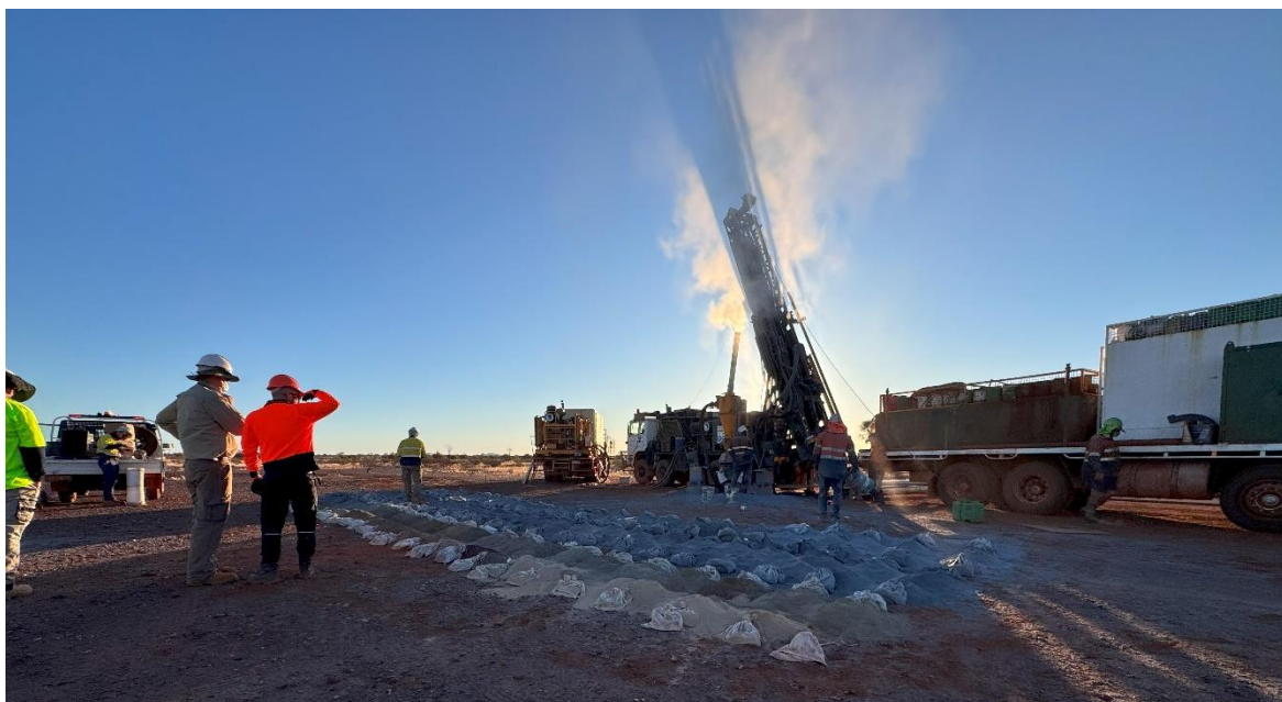
Figure 1: Reverse circulation (RC) drill rig at Dante Project.
