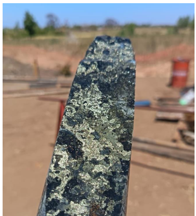
Figure 3: MPYDD001: Sulphide alteration in NQ core at a depth of 85m downhole. Drilling and sampling of MPYDD001 (Anomaly Target 2) ongoing at the time of reporting.
