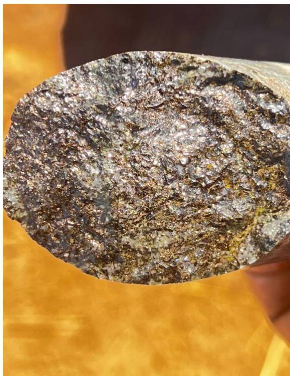
Figure 3: MPYDD001: Sulphide alteration in NQ core at a depth of 85m downhole. Drilling and sampling of MPYDD001 (Anomaly Target 2) ongoing at the time of reporting.
