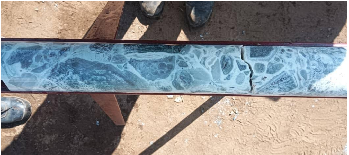
Figure 2: Breccia occurring at 188m(downhole) at Drill hole MPODD004. Sampling and assaying of MPYDD004 (Anomaly Target 1) ongoing at the time of reporting.
