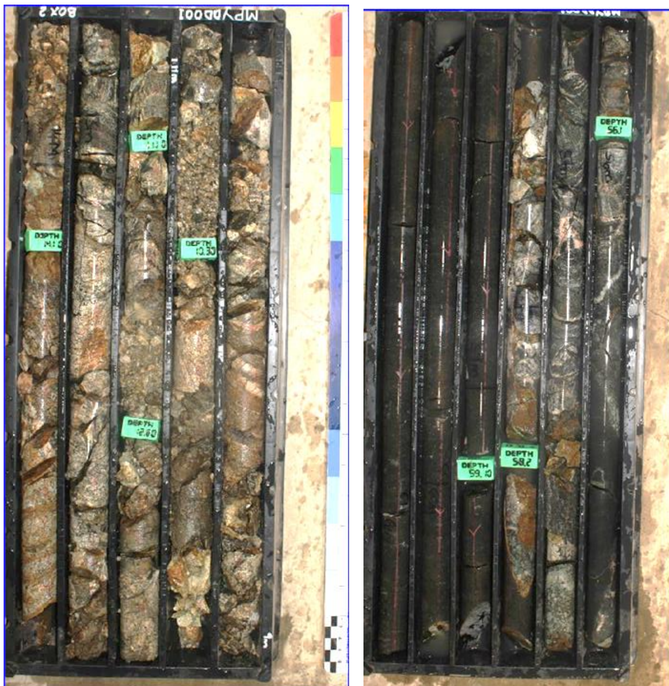
Figure 9 ; Mpyupyu anolmaly drillhole MPYDD001- (Left) Potassic alteration (fenitisation) and brecciation of wall rock adjacent intrusive system (9.3 to 14.3m downhole), Right - Barite rich dyke or stringer at 57 to 58 m down hole indicating increased sulphide activity. Drilling and sampling of MPYDD001 (Anomaly Target 2) ongoing at the time of reporting.
