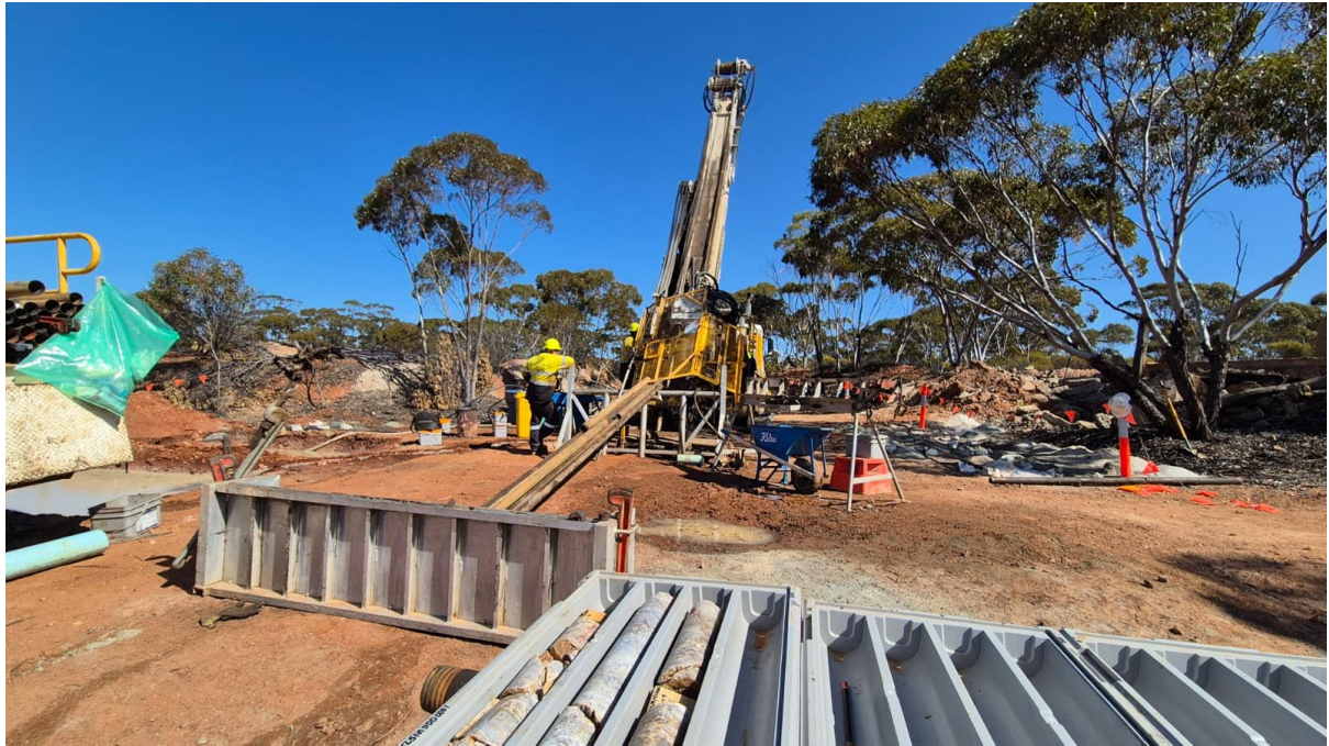
Figure 2: Diamond core drilling underway at the Mt Palmer Gold Project.
