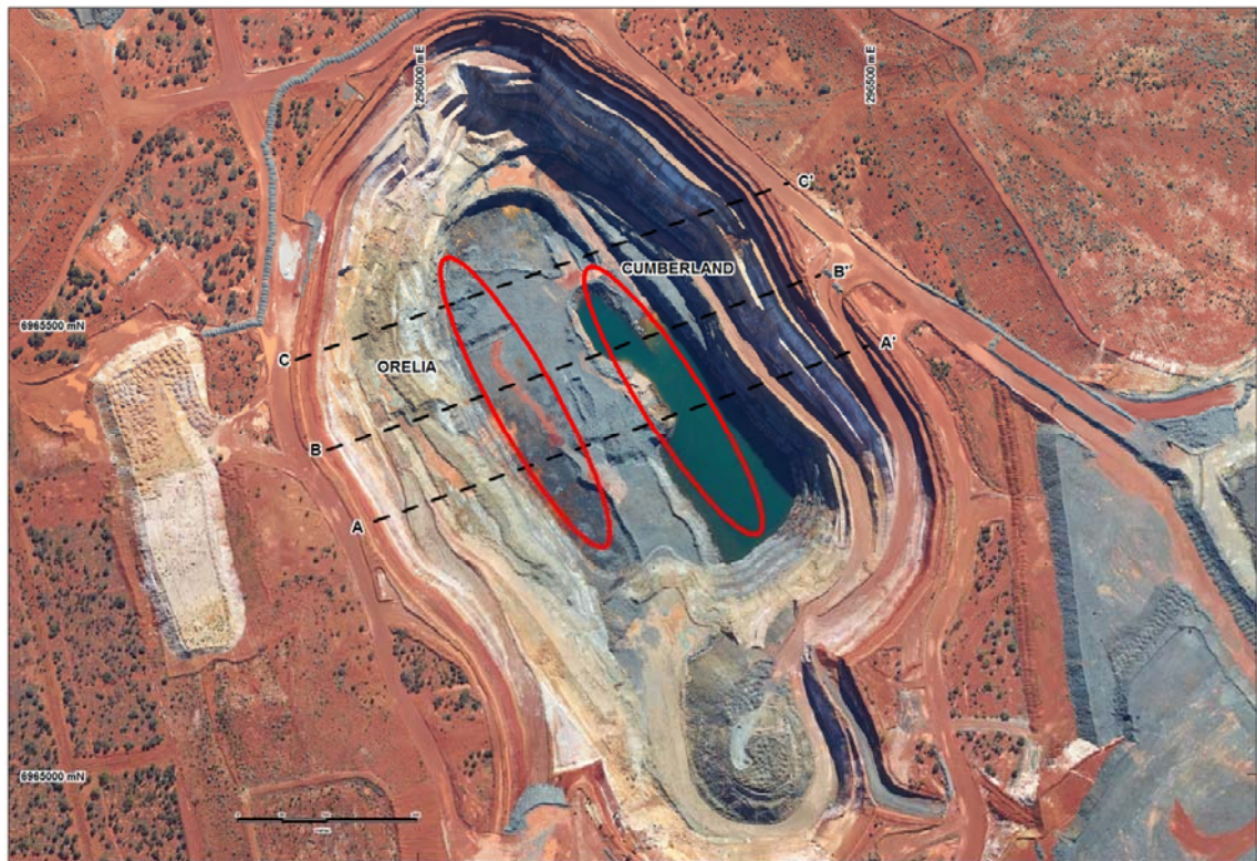
Figure 3: Cockburn image showing location of sections, Orelia and Cumberland ore zone
